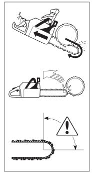
In this case the saw pulls itself towards the tree and the front edge of the saw provides a natural rest when cutting. Cutting on the pull stroke gives you better control over the saw and the position of the kickback zone.
